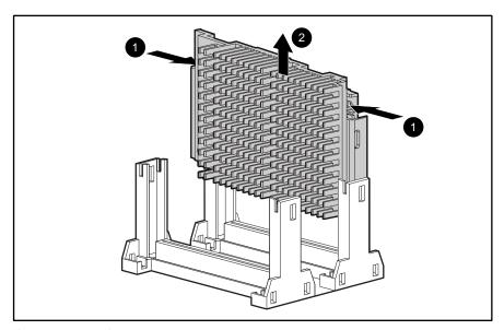
Figure 2-31. Removing a processor
